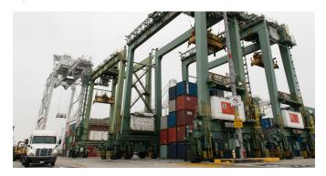
**Rubber tire gantry cranes:** Diesel-powered gantry cranes, which are used to move shipping containers, were electrified. These machines have been identified as the second largest source of nitrogen oxide (NOx) emissions at the terminal.
