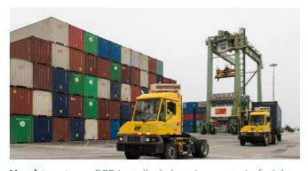
**Yard tractors:** SCE installed charging ports in freight yards to transition the tractors that move shipping containers around the port facility from diesel to zero-emission electricity.
